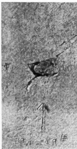
Fig. 2—Same area after 5-minute etch in hot dilute HCl.
